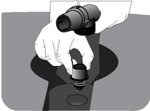
Turn the Trough upside down, press the Kiwitech valve into position and screw the Trough Tee into place so that it is a firm fit and aligns with the axis of the tunnel.
