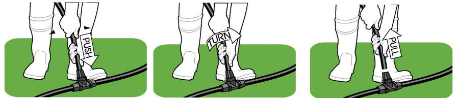
Unplug the trough lead from the hydrant. With one foot on the pipe and hydrant to hold it steady “Push, twist anti-clockwise, pull back”
