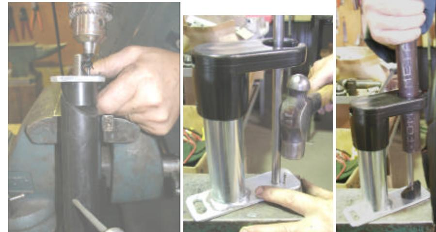
**VP STYSUPD:** PP Stylus Double Support - lower Stylus plastic drilled, pin/Stylus fitted & aligned + XHEX 10-25Z
