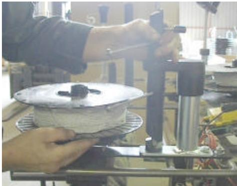
If the Roller Arms run under the Spool flange or way above it, then the only thing we can do is to bend the Roller Arms up or down until they run over the Spool nicely. This is not ideal, but, the only fix in this instance.
