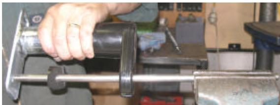
After drilling, release the tension on the Ball Detent System by undoing the Grub Screw a bit. Remove the Stylus Middle and Bottom Plastic.
