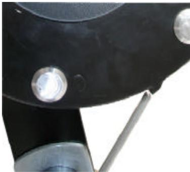
Move the Stylus around into "Locked" position and tap the Base Drive Plate down until it touches the top of the Stylus Lock. Mark where the Lock Arm needs cutting in order to engage the Base Drive Plate Stop perfectly.
