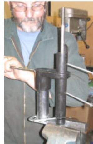
Thread the “assembled” Stylus Middle (Double or Triple) onto the Stainless Steel Rod and turn the Stylus to “On” indexed position (i.e. when the Roller Arms would be sitting on Spools). Position the Stylus Plastic Bottom so that it meets nicely with the Stylus Middle (i.e. so the two are “mated”). Tighten the Grub Screw.
