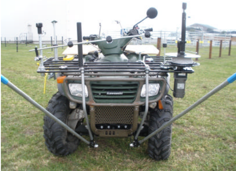
Figure 10: Finished product (much of the PowerPac's weight now resting on the strong quad frame)
