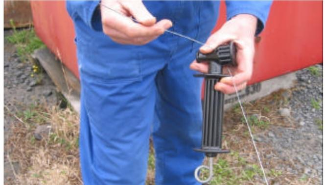
Step 2: Bend wire 'end' out of the way (towards small drum of Handle Strainer).
