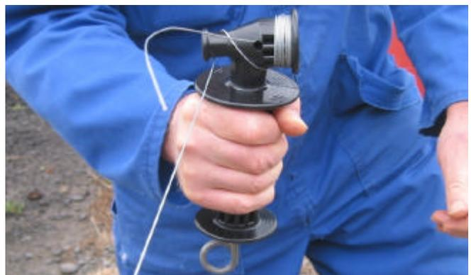
Step 6: When the large drum end of the Handle Strainer is 5cm from pulling up alongside the 'hook on point' of the Kiwitech or homemade thong take the wire over to the small drum.
