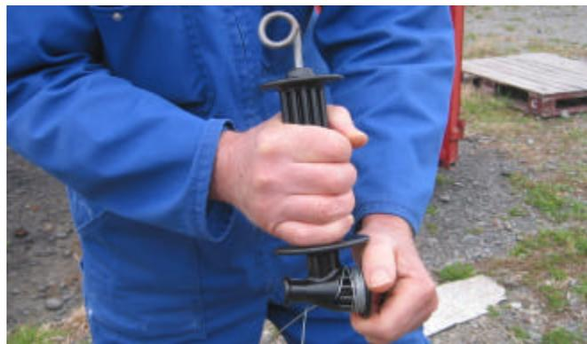
Step 5: Wind on enough wire to suit anticipated 'spare' requirements (the big drum was designed to be a wire reservoir to add length to the fence i.e. after fixing a number of breaks).
