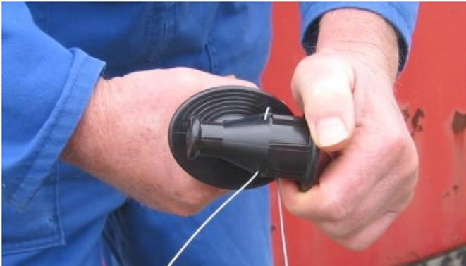
Step 3: Begin to wind wire (under tension for a tight wrap) around the big drum of the Handle Strainer.
