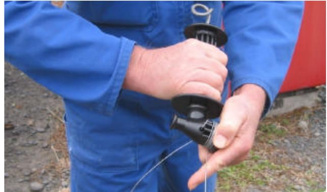
Step 4: Use hand and index finger as a brace when rotating Handle (also helps guide wrap).
