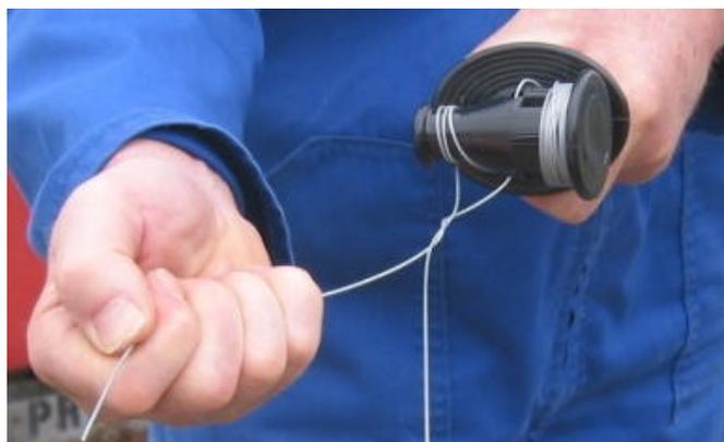
Step 10: Once tension has been decided, take the wire 'end' and 'lazy wrap' around the tensioned length. Finish off by kinking end.
